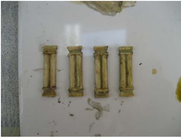
14 - Epoxy castings after colouring (original far left + 3 duplicates)
