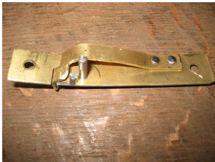
16 - Newly fabricated lock
